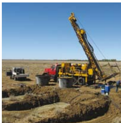
Diamond drill rig, Levuka
